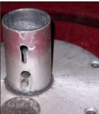
Drill and file holes into the tube for where the seat base locks, since I cut that part off. The bottom of the pedestal has more problems to deal with than the top part. Brian bought a new base and he mounted a oblong 1/4 inch aluminum diamond plate to his boat floor. This is to help spread the load, cover the hole from where his aluminum base was removed and relocated his seat a little rearward. The suspension system does move
