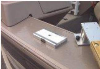
Mounting the reels was really quite simple; I just placed a 6" universal mount from Bert's Custom Tackle just behind the console on both sides of the boat. Bert also makes an "L" shaped handlining reel mount that clamps into the universal when needed, but can be easily removed when jigging, trolling or boat riding if your wife is anything like mine.
